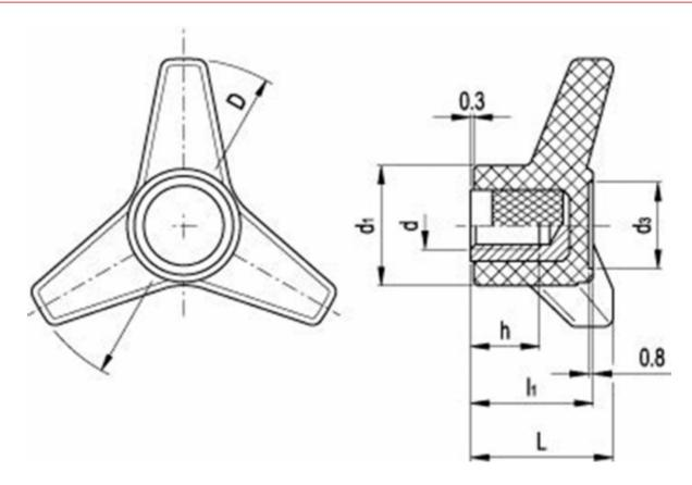
$\begin{array}{lll} D & = 130 \\ d1 & = 43 \\ d3 & = 29 \\ dh & = M16 \\ h & = 22 \\ I1 & = 40 \\ L & = 47 \\ Weight in (g) = 164 \\ \end{array}$
